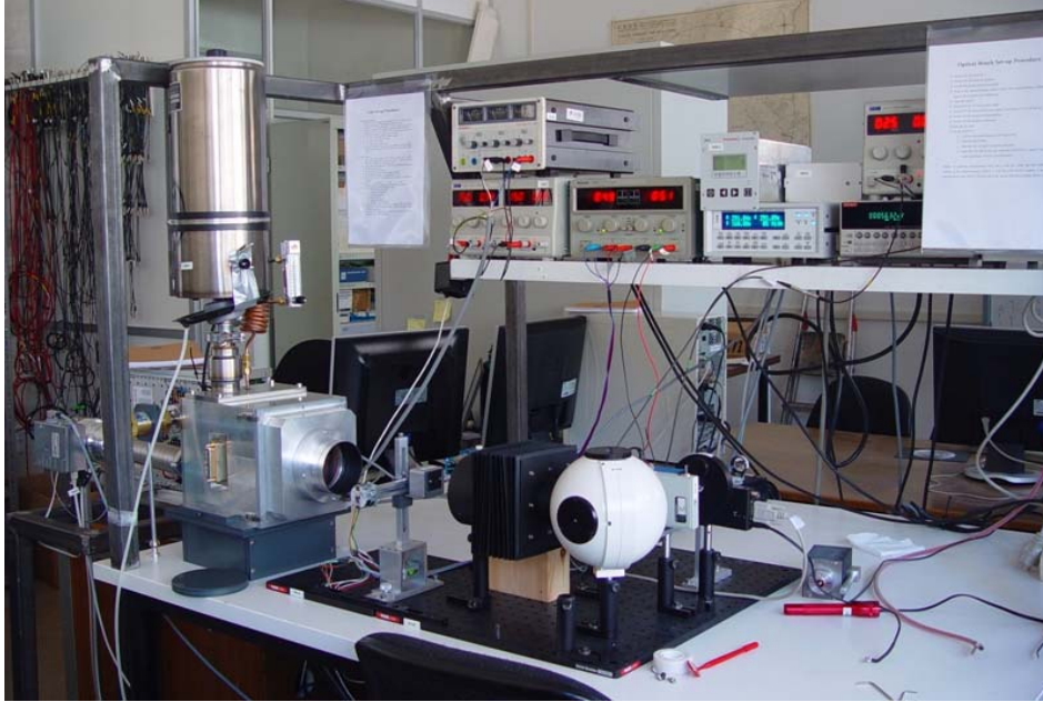
A photograph of the test bench for the DES electronics. To the left of the picture one can see the cube that contains the CCD, together with a small liquid nitrogen Dewar, to maintain it cold. On the right there is an optical system to illuminate the CCDs. The electronics are inserted in a crate in the back of the picture (not seen).
