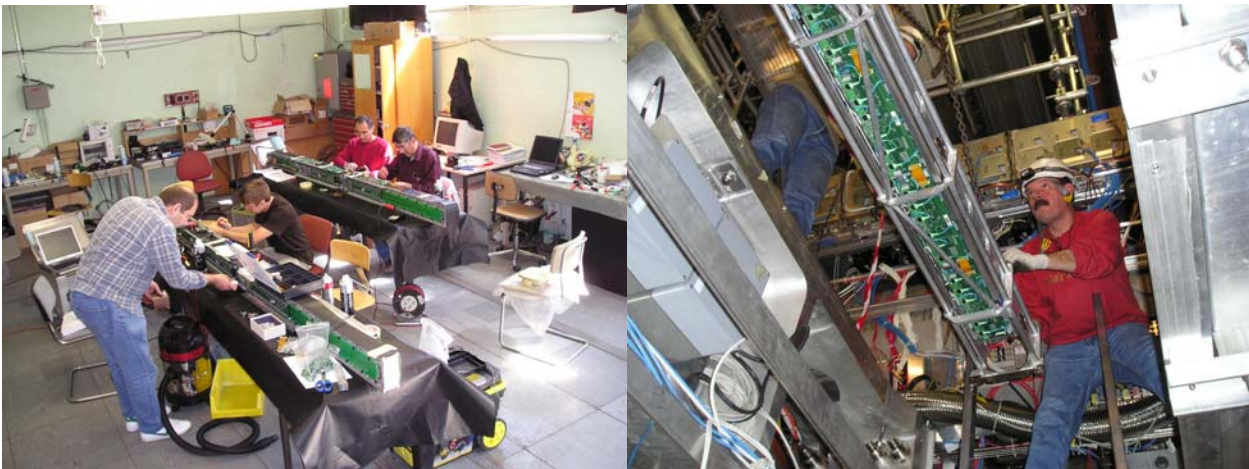
A small part of the Tilecal drawers were refurbished on the surface outside the ATLAS cavern. The refurbishment process is shown on the right, while the drawer insertion in the Tilecal module, using the insertion tool produced at IFAE, is shown on the left
