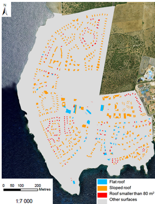
Fig. 3. Digitization of the touristic hub of Cap d'Artrutx: identification of the type of roof for evaluating the photovoltaic potential.
