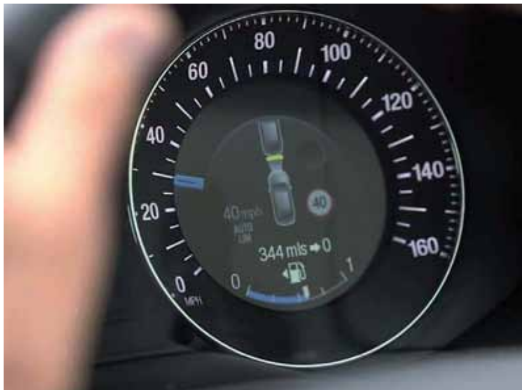
The image – captured from the new film made by ETSC – shows Intelligent Speed Adaptation (ISA) technology in the form of a speedometer that is currently used in many models of cars.
